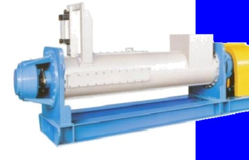
For the process de-inking or pulp bleach. This system was designed to mix and penetrate the chemicals uniformly for effect of chemicals.
